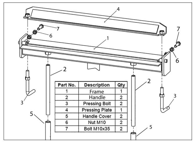
Mount the Metal Folder in a vice, at a height which allows easy operation taking into account the nature of the work with the handles pointing towards you.
